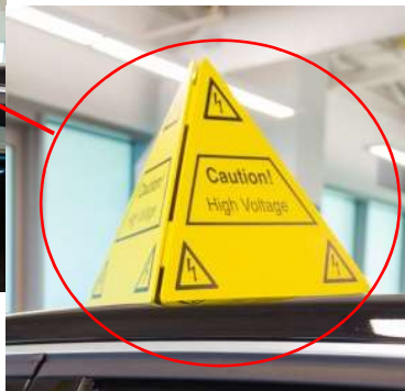
Marking of HV vehicle in workshop
